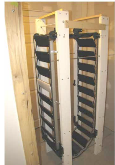
Figure 114: An air flow regulator that provides resistance by recovering air flow energy by using moving blading to drive an electrical generator
